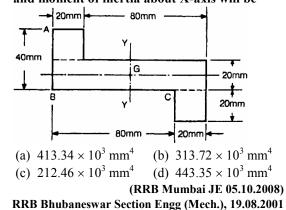
Ans. (a) : Section is symmetric about x-axis & y-axis so distance of centroid G from AB =  $\frac{20+80}{2}$  = 50 mm Height of centroid G from BC =  $\frac{20}{2}$  = 10 mm Now moment of inertia about X-X of cross section  $I_{XX} = \frac{100 \times 20^3}{12} + 2 \left[ \frac{20 \times 20^3}{12} + (20 \times 20) \times 20^2 \right]$ = [6.667 + 34.667] × 10<sup>4</sup> = 413.34 × 10<sup>3</sup> mm<sup>4</sup>
