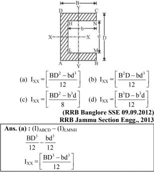
149. What is the value of moment of inertia of Tsection about centre of gravity through X-X and Y-Y axis, given figure below.
