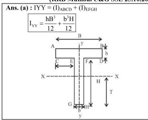
150. What is the value of moment of inertia of Lsection about centre of gravity through X–X and Y–Y axis, given figure below.
