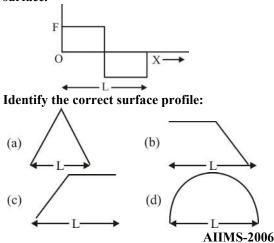
**Ans. (a) :** The figure shows that the force is constant during loading and unloading. In figure (b) and (c) there are regions of constant slope. Thus no force is required in loading through those regions. But the force always has a magnitude. In figure (d), the force needs to change at every point as the inclination of the surface change at every point.]
