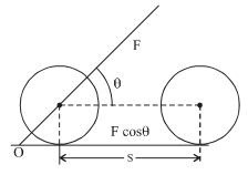
Work is a scalar quantity. Its SI unit is joule. One joule is defined as the amount of energy exerted when a force of 1 newton is applied over a displacement of one metre.
