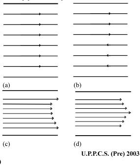
In a streamlined motion, the speed of layers of liquid is lowest near the pipe. As moved away from the pipe, the motion of layers gradually increases.
